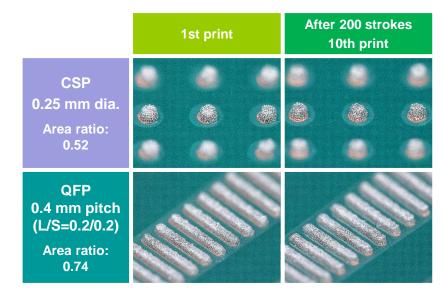
Area ratio =  $\frac{\text{Aperture area}}{\text{Aperture wall area}}$
