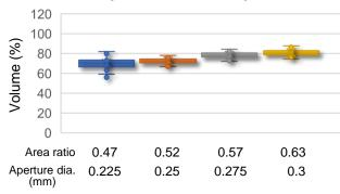
➤ Consistent paste transfer volume from the initial paste print even after 60 min. pause even with area ratio ≥0.52.
