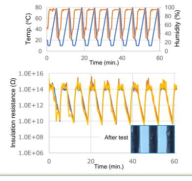
➤ S3X58-HF1100-3 showed robust high reliability under harsh conditions, with no evidence of dendrite growth observed.
