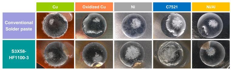
➤ Newly developed powerful activator technology provided excellent solder spreading not only on standard substrates, but also difficult to solder oxidized Cu, C7521 & Al/Ni substrates.
