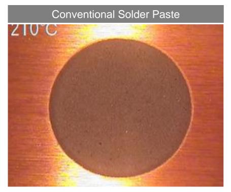
Flux splatters on the glass plate as the flux and generated gas inside molten solder evacuate.
