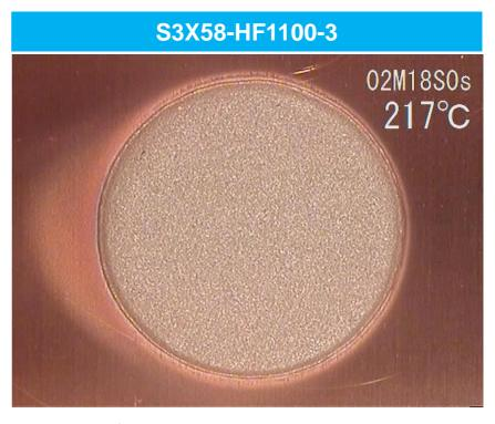
Instant flux and gas evacuation prevents flux splattering.
