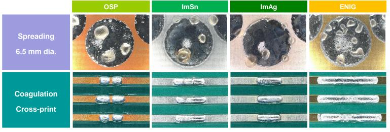
> Regardless of the type of surface finish, the solder spread well and no solder balls were left inbetween tracks after coagulation.
