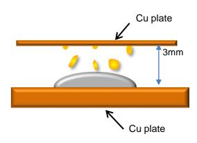
Place Cu plate above deposited solder paste and reflow to allow for attachment of flux splatter.
