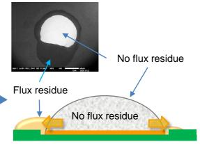
Flux residue swiftly coagulate as solder melts leaving none on either top or inside of the fillet
