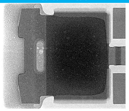
Test board: In-house design, OSP Component: PwTr (Sn plating)
