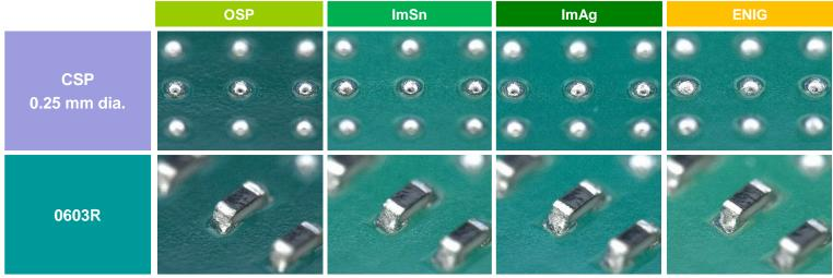
> Regardless of the type of surface finish, the solder coalesced completely and caused no unmolten solder particles.
