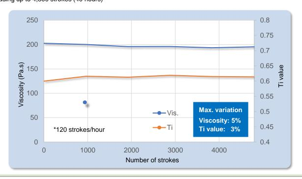
➤ Continual paste print strokes with periodical paste replenishment resulted in stable rheology (viscosity and thixotropy).
