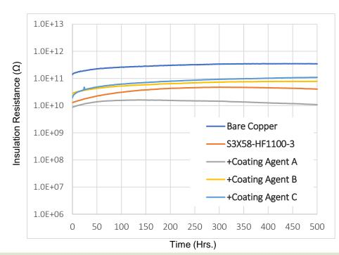
> With or without conformal coating applied, S3X58-HF1100-3 had high insulation resistance.
